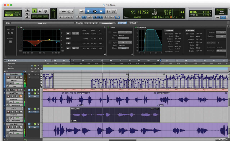
The new Channel Strip features a four-band EQ, filters, and compressor/limiter.
